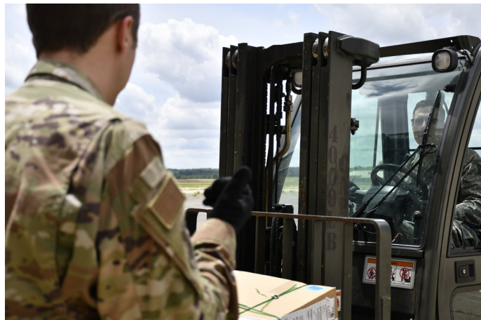
Senior Airman David Parks, 110th Force Support Squadron services personnel, uses standardized hand-and-arm signals to guide his counterpart, Tech Sgt. Trent Wollberg in lifting, moving, and placing a palletized load during training.
